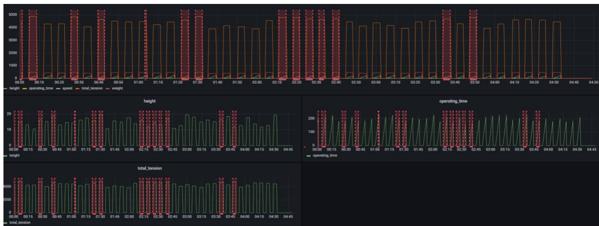
Figure 8.1. Grafana-based visualisation of anomaly intervals in the load-unload operation detected after GAA ran on the gateway.
