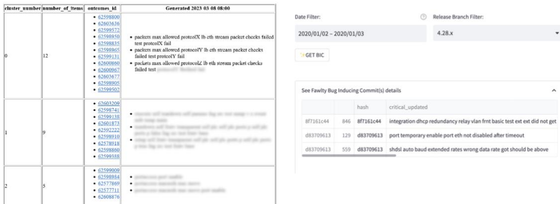
Figure 63 Tools from RISE. LogGrouper (left) clusters failing tests based on similarities in log files from test execution. BugIdentifier Tool (right) proposes code changes that could have caused failing tests
